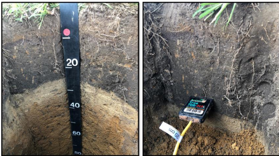
Figure 3. Borehole for soil sensor installation with tape (left) and sensor inserted (right). Note that soil horizons that vary in soil color, texture, and structure. A soil scientist can help describe this profile. This information can be useful for stakeholders for interpreting soil moisture data measured in the soil profile. Image Credit: Matthew R. Levi, University of Georgia.
