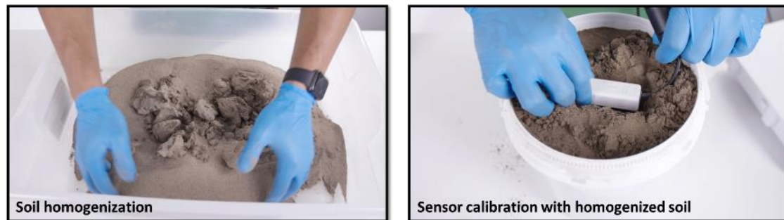
Figure 5. Sensor calibration in lab. Image Credit: Leo Rivera.
